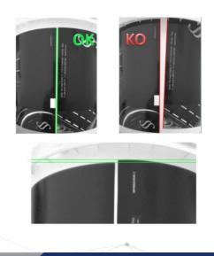
Automatic check for in molding labeling correct size and positioning
